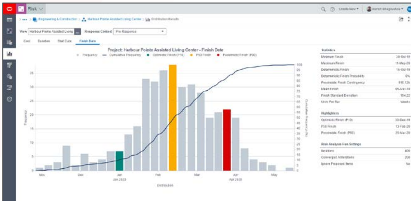
Figure 8. Monte Carlo-based histograms provide likely project outcomes based on potential risk, not just the planned schedule.
